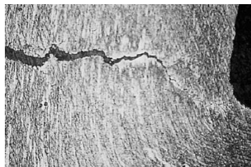
Figure 4: Micrograph of the Weld & Heat Affected Zone of a C-Ring Specimen
