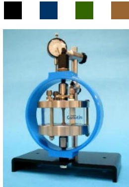
Figure 1: NACE Proof Ring, used for performing SCC/EAC tests per TMO 177 1
