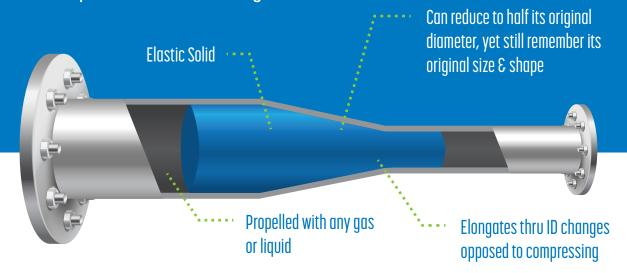
ElastiPig is a highly malleable, elastomer-solid pig that exerts minimal outward pressure when transitioning flowlines. It creates 100% surface area contact with the pipe wall, providing excellent sealing capabilities. ElastiPigs are useful when used alone or in combination with mechanical pigs, pipeline gels and/or chemicals.
