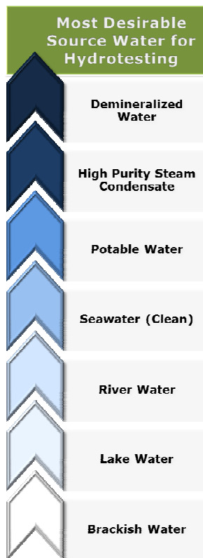
Figure 1: General Ranking of Water Sources for use in Hydrostatic Testing
