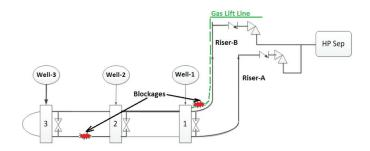
A West Africa field operator witnessed an abnormal increase in pressure topsides when the flowline circulation pump was used to pump dead oil into the production line. No increase in subsea pressure was observed. Operational history prior to blockage hinted at the possibility of the presence of one or both wax and hydrate blockages in the production line. Depressurization options were limited by the blocked gas lift line.
