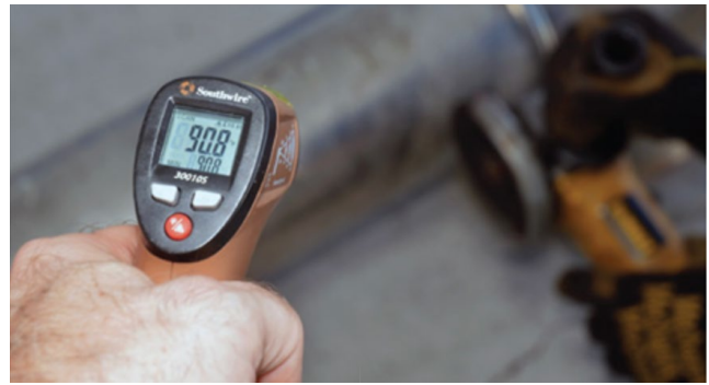
Figure 4. A non-contact infrared thermometer can be useful for measuring temperatures.
